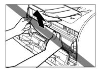
7 Gently pull the jammed paper between the output rollers until the leading edge emerges from the machine.
